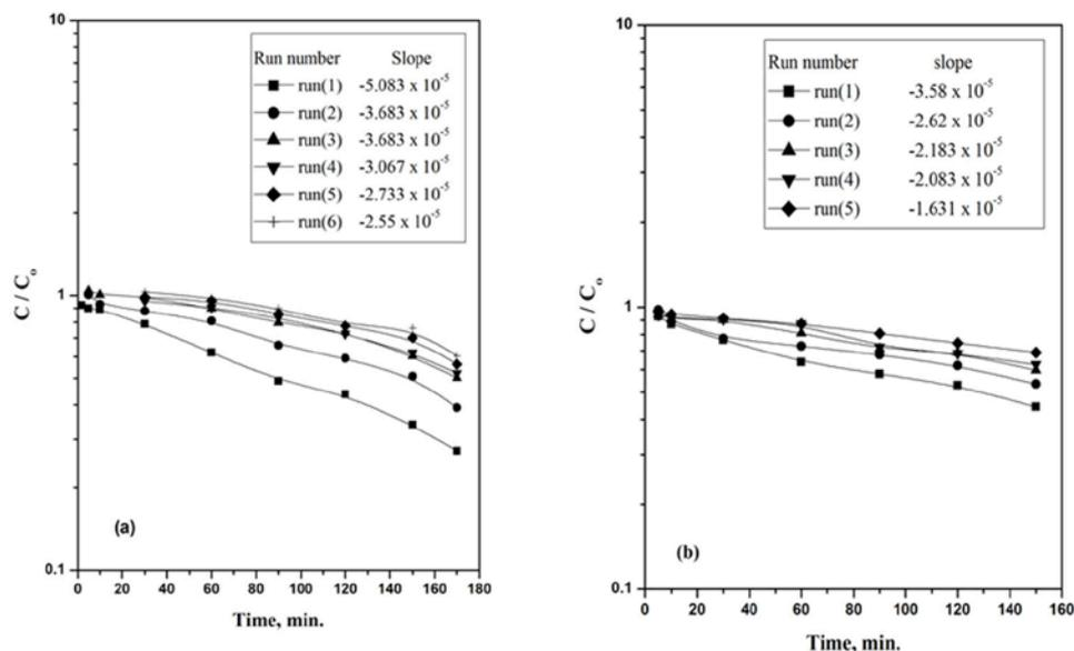
Figure 9: Effect of time on the transfer of Zn(II) through SLM impregnated with CYANEX 925 in kerosene under the optimum conditions of Zn(II) transfer for five runs: (a) without Co(II), (b) with Co(II). ( $[Zn(II)] = 0.005$  M,  $[NH_4SCN] = 0.1$  M,  $[H_2SO_4] = 0.01$  M,  $[Co(II)] = 0.005$  M,  $[Na_2SO_4] = 0.49$ M,  $[NH_3]_{Soln.} = 3$ M,  $[CYANEX 925] = 0.025$  M,  $[H^+] = 0.01$ ).
