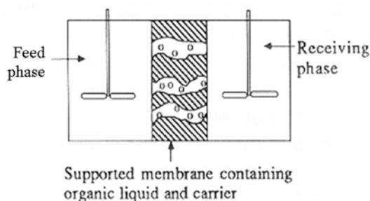
Figure 1: Thin sheet supported liquid membrane.
