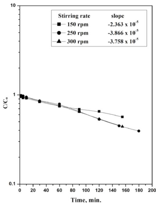
Figure 2: Effect of stirring rate on the transfer of Zn(II) through SLM in the aqueous mixed sulphate and thiocyanate solutions ( $[Zn(II)] = 0.005$  M,  $[NH_4SCN] = 0.1$  M,  $[H_2SO_4] = 0.01$  M,  $[H^+] = 0.01$ ,  $[Na_2SO_4] = 0.49$  M,  $[NH_3]$  Soln. = 1 M,  $[CYANEX\ 925] = 0.015$  M).
