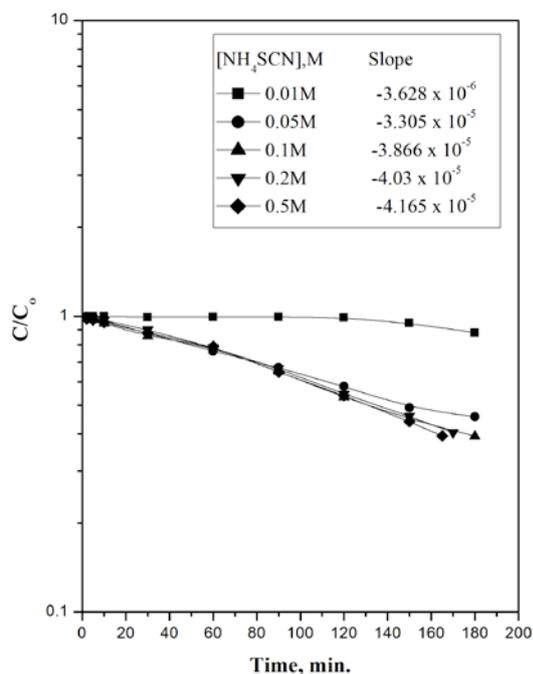
Figure 6: Effect of  $\text{NH}_4\text{SCN}$  on the transfer of Zn(II) through SLM impregnated with CYANEX 925 in kerosene from the aqueous mixed sulphate and thiocyanate solutions ( $[\text{Zn(II)}] = 0.005 \text{ M}$ ,  $[\text{CYANEX 925}] = 0.015 \text{ M}$ ,  $[\text{H}_2\text{SO}_4] = 0.01 \text{ M}$ ,  $[\text{H}^+] = 0.01$ ,  $[\text{Na}_2\text{SO}_4] = 0.49 \text{ M}$   $[\text{NH}_3] \text{ Soln.} = 1 \text{ M}$ ).
