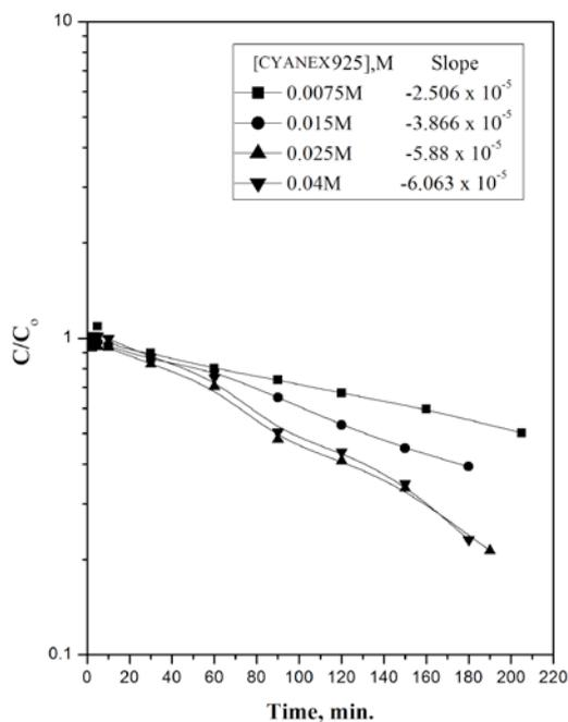
Figure 3: Effect of CYANEX 925 concentration on the transfer of Zn(II) through SLM from the aqueous mixed sulphate and thiocyanate solutions ( $[Zn(II)] = 0.005$  M,  $[NH_4SCN] = 0.1$  M,  $[H_2SO_4] = 0.01$  M,  $[H^+] = 0.01$ ,  $[Na_2SO_4] = 0.49$  M,  $[NH_3]$  Soln. = 1 M).
