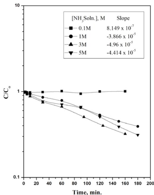
Figure 7: Effect of ammonia solution concentration on the transfer of Zn(II) through SLM impregnated with CYANEX 925 in kerosene from the aqueous mixed sulphate and thiocyanate solutions ( $[\text{Zn (II)}] = 0.005 \text{ M}$ ,  $[\text{NH}_4\text{SCN}] = 0.1 \text{ M}$ ,  $[\text{H}_2\text{SO}_4] = 0.01 \text{ M}$ ,  $[\text{H}^+] = 0.01$ ,  $[\text{Na}_2\text{SO}_4] = 0.49 \text{ M}$ ,  $[\text{CYANEX 925}] = 0.015 \text{ M}$ ).
