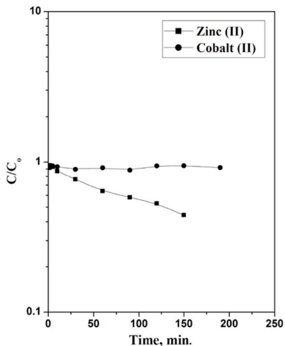
Figure 8: Effect of time on the transfer of metal ions through SLM impregnated with CYANEX 925 in kerosene from its admixture under the optimum conditions of Zn(II) transfer ( $[Zn(II)] = 0.005$  M,  $[NH_4SCN] = 0.1$  M,  $[H_2SO_4] = 0.01$  M,  $[H^+] = 0.01$ ).
