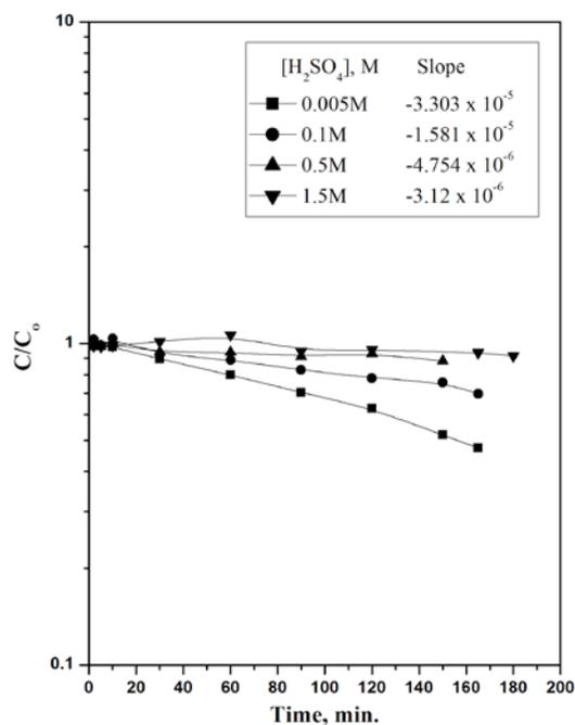
Figure 5: Effect of H<sub>2</sub>SO<sub>4</sub> concentration on the transfer of Zn(II) through SLM impregnated with CYANEX 925 in kerosene from the aqueous mixed sulphate and thiocyanate solutions ([Zn (II)] = 0.005 M, [NH<sub>4</sub>SCN] = 0.1 M, [CYANEX 925] = 0.015M, [NH<sub>3</sub>] Soln. = 1M).
