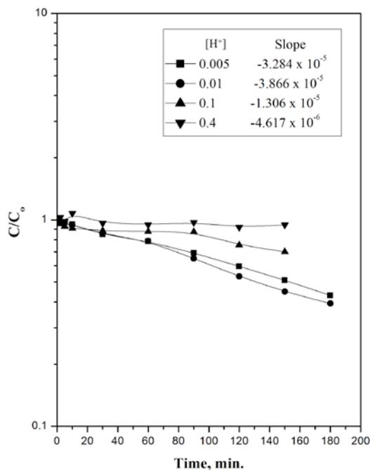
Figure 4: Effect of hydrogen ion concentration on the transfer of Zn(II) through SLM impregnated with CYANEX 925 in kerosene from the aqueous mixed sulphate and thiocyanate solutions ( $[Zn(II)] = 0.005$  M,  $[NH_4SCN] = 0.1$  M,  $[CYANEX 925] = 0.015$  M,  $[NH_3]$  Soln. = 1 M).
