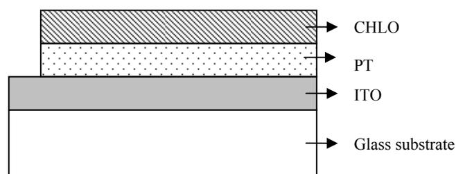
Figure 1: The layer of thin film sample of ITO/PT/CHLO *p-n* heterojunction solar cell.
