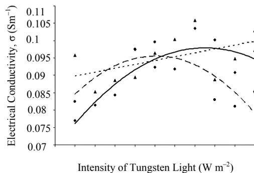
Figure 6: Electrical conductivity of PT5/CHLO thin films under illumination with different thicknesses of CHLO thin films. — CHLO 5; - - - CHLO 7; ..... CHLO 10.
