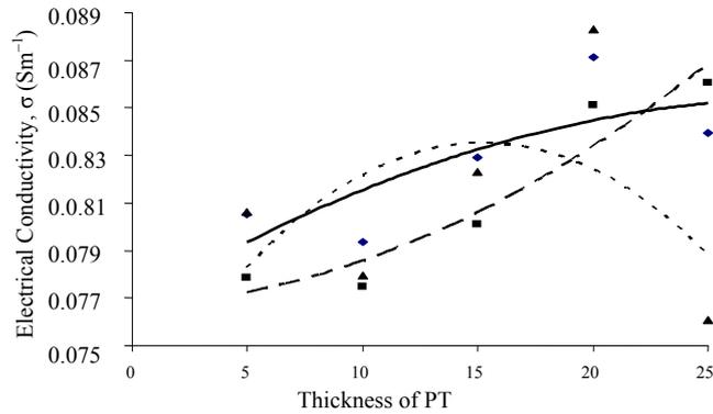
Figure 4: Electrical conductivity of PT/CHLO thin films at different thicknesses of PT. — CHLO 5; - - CHLO 7;..... CHLO 10.
