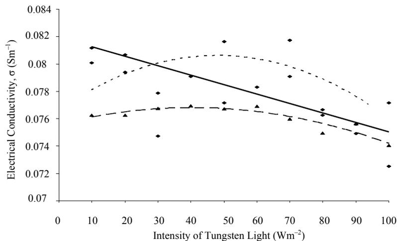
Figure 9: Electrical conductivity of PT20/CHLO thin films under illumination with different thicknesses of CHLO thin films. — CHLO 5; - - - CHLO 7; ..... CHLO 10.
