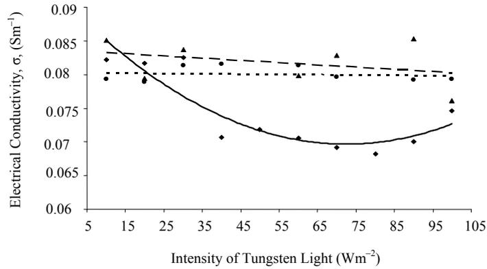
Figure 7: Electrical conductivity of PT10 thin films under illumination. PT10 with different thicknesses of CHLO thin films. — CHLO 5; - - - CHLO 7, ..... CHLO 10.
