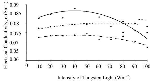
Figure 8: Electrical conductivity of PT15/CHLO thin films under illumination with different thicknesses of CHLO thin films. — CHLO 5; - - - CHLO 7; ..... CHLO 10.
