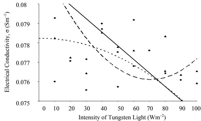
Figure 10: Electrical conductivity of PT25/CHLO thin films under illumination with different thicknesses of CHLO thin films. — CHLO 5; - - - CHLO 7; ..... CHLO 10.
