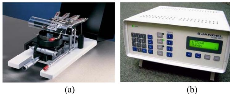
Figure 2: The four point probes instrument consists of (a) Jandel Universal Probes and (b) Jandel RM3 Test Unit as a control current and so on.
