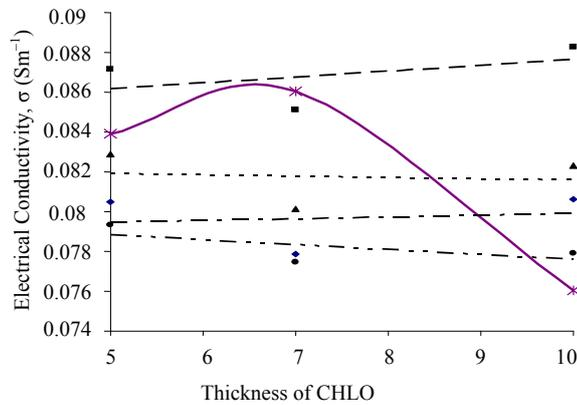
Figure 5: Electrical conductivity of PT/CHLO thin films at different thicknesses of CHLO. — · — PT5; - - · - PT10; ..... PT15; - - - PT20; — PT25.
