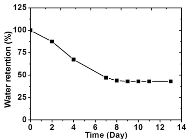
Figure 5: Effect of standing time of SAP on water retention (CMC/AAC = 1.0:1.5, room temperature = 27°C, dose = 5 kGy).
