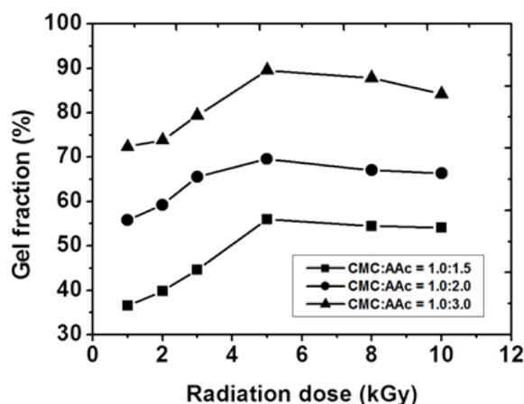
Figure 2: Effect of radiation dose and concentration of AAc on gel fraction of CMC/AAc SAP.
