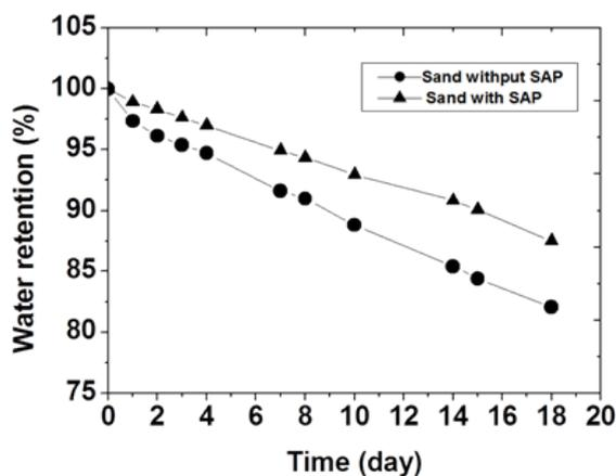
Figure 6: Effect of standing time of SAP in sand on water retention (CMC/AAC = 1.0:1.5, room temperature = 27°C, dose = 5 kGy, SAP = 1%).
