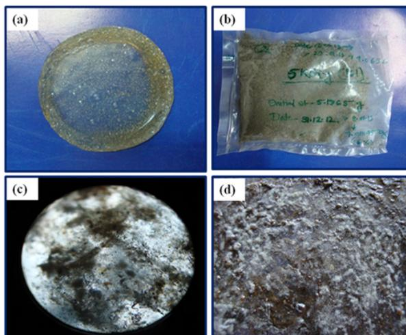
Figure 10: Biodegradation of SAPs film (a) before degradation, (b) compost bed for degradation, (c) degraded SAP after three weeks in a swollen state and (d) after four weeks in a dried state.
