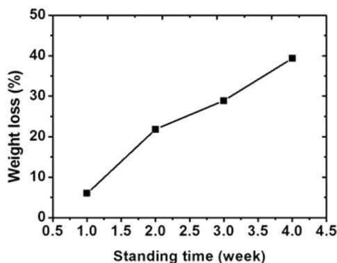
Figure 9: Effect of standing time of SAP in compost environment on degradation.
