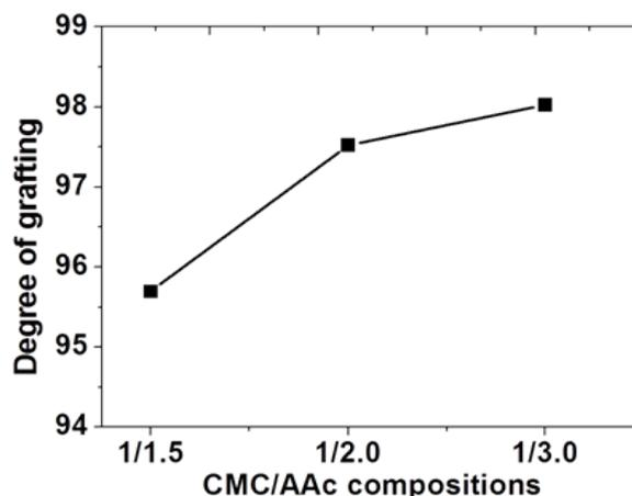
Figure 3: Effect of concentration of AAc in CMC/AAc SAP on degree of grafting at 5 kGy radiation dose.
