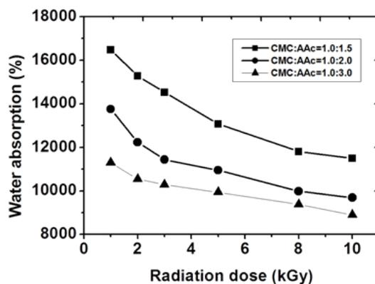
Figure 4: Effect of radiation and concentration of AAC on water absorption of CMC/AAC SAP.
