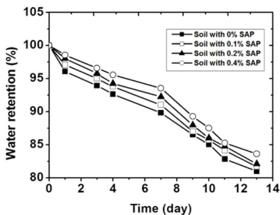
Figure 7: Water retention of soil with 0%, 0.1%, 0.2% and 0.4% SAP (CMC/AAC = 1.0:1.5, room temperature = 20°C, dose = 5 kGy).
