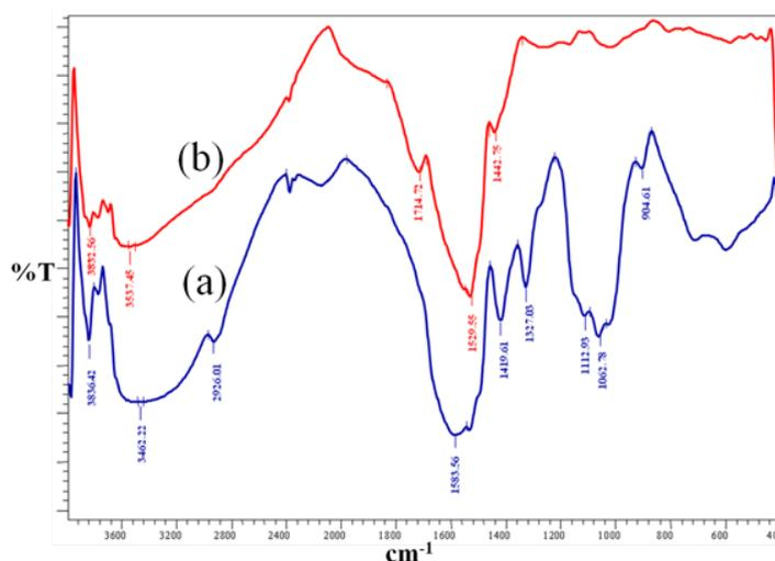
Figure 1: Infrared spectroscopy of (a) CMC powder (blue colour spectrum) and (b) SAPs of CMC/AAc (red colour spectrum).
