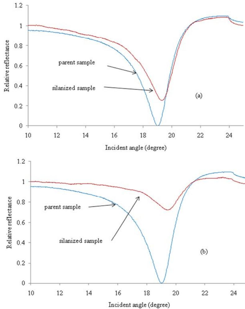
Figure 2: Reflectivity versus incident angle for a 50 nm thin silver film (black line) silanised with APTES (gray line) by CVPD method at 100°C (a) and by DVPD method at 80°C (b) for 30 min.
