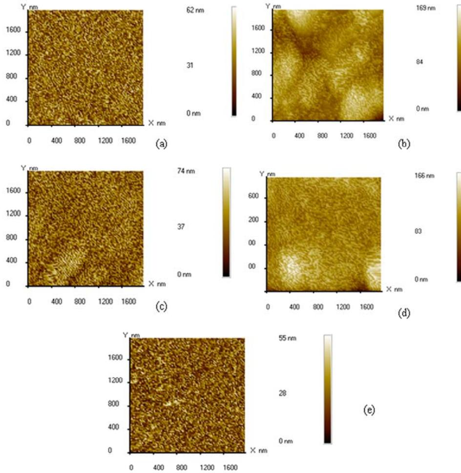
Figure1: AFM images of (a) sputtered 50 nm thin silver film; (b) silanised with APTES by CVPD method at 100°C for 60 min; (c) silanised with APTES by CVPD method for 30 min at 80°C; (d) by DVPD method at 100°C for 60 min; and (e) by DVPD method for 30 min at 80°C.
