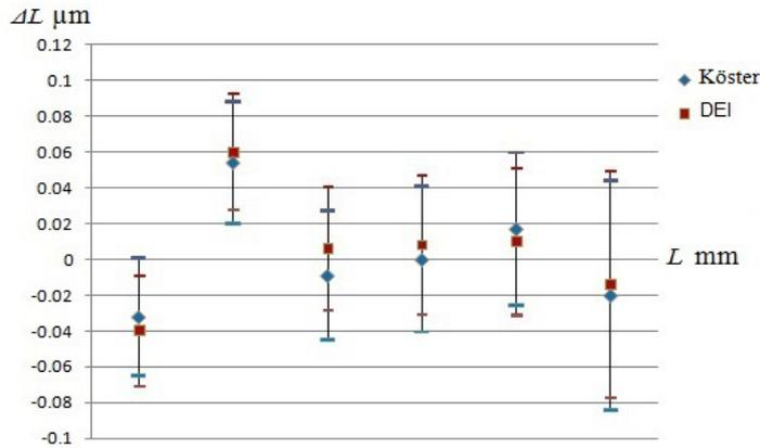
Figure 6: Results obtained by the DEI and Köster comparator for a set of 6 gauge blocks of length (2 mm, 5 mm, 10 mm, 20 mm, 25 mm, and 75 mm) show good agreement.
