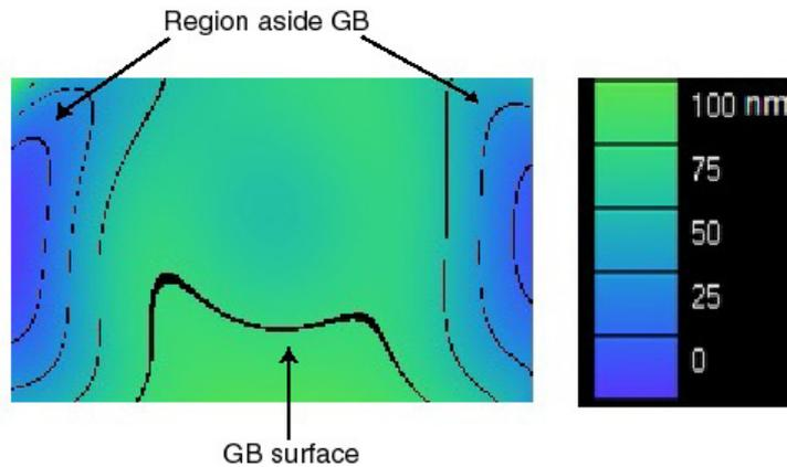
Figure 4: Surface mapping of gauge block and the aside region.
