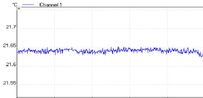
Figure 5: Gauge block's temperature display for 3 h shows good stability of the gauge block in the interferometer.
