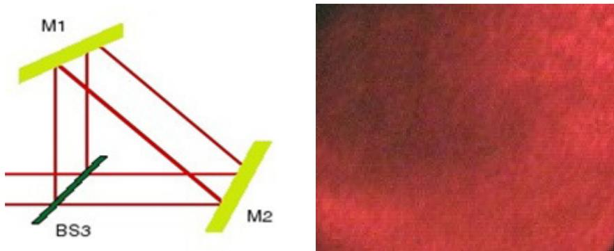
Figure 2: One pattern is observed in the interference region between the opposite mirrors at the measurement arm (M1, M2) in the absence of gauge block.
