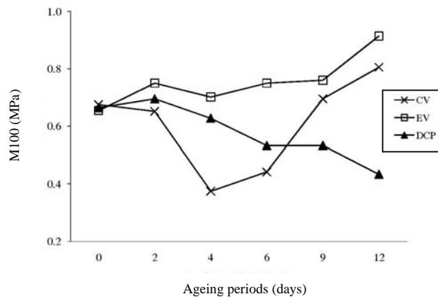
Figure 1: Tensile modulus values of natural rubber cured with CV, EV and DCP curing systems before and after ageing for 2, 4, 6, 9 and 12 days at 100°C.
