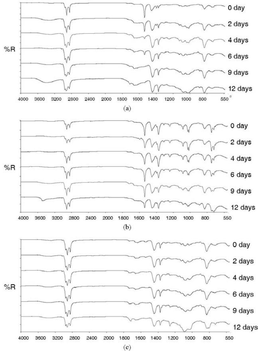
Figure 6: FTIR analysis measurements of natural rubber cured with CV, EV and DCP curing systems before and after ageing for 2, 4, 6, 9 and 12 days at 100°C, which are (a) CV, (b) EV and (c) DCP curing systems.
