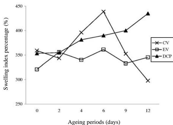
Figure 5: Swelling index percentages of natural rubber cured with CV, EV and DCP curing systems before and after ageing for 2, 4, 6, 9 and 12 days at 100°C.
