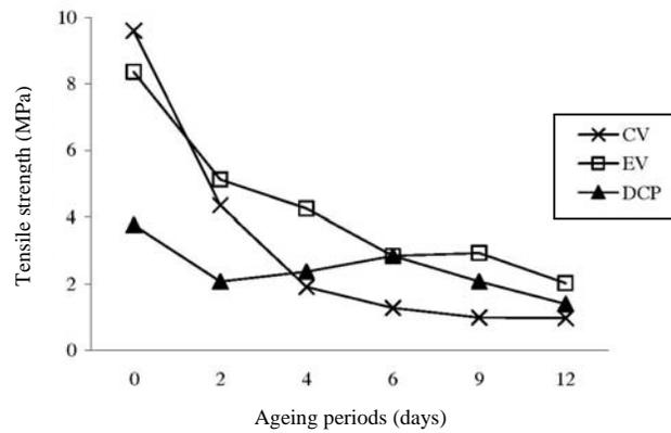
Figure 4: Tear strength values of natural rubber cured with CV, EV and DCP curing systems before and after ageing for 2, 4, 6, 9 and 12 days at 100°C.
