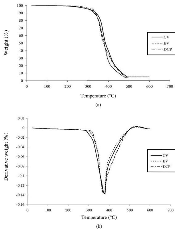
Figure 7: (a) TGA and (b) DTG curves of natural rubber cured with CV, EV and DCP curing systems.
