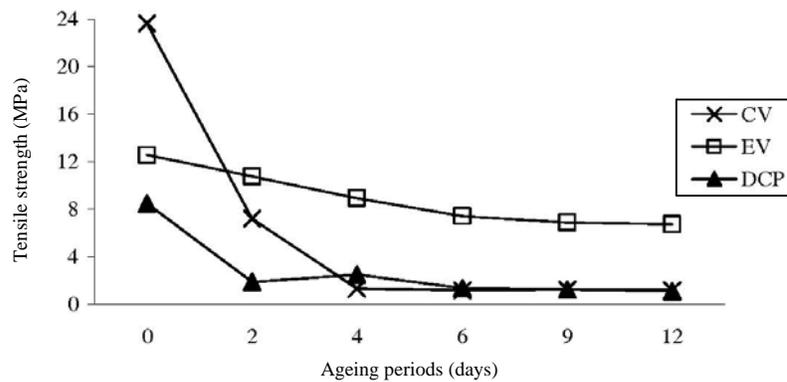
Figure 2: Tensile strength values of natural rubber cured with CV, EV and DCP curing systems before and after ageing for 2, 4, 6, 9 and 12 days at 100°C.
