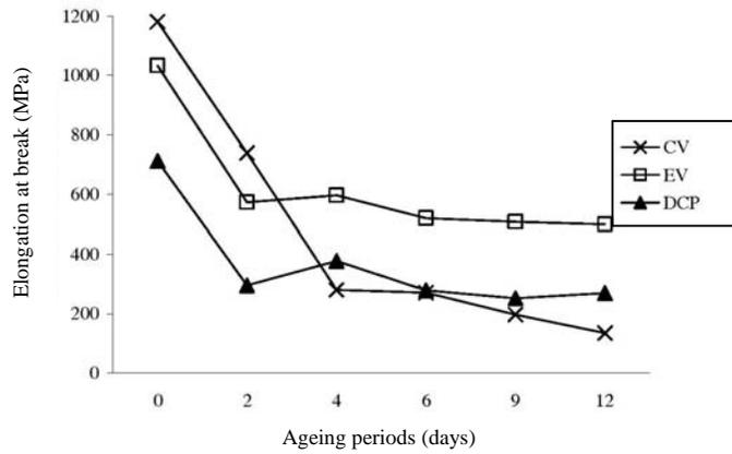
Figure 3: Elongation at break percentages of natural rubber cured with CV, EV and DCP curing systems before and after ageing for 2, 4, 6, 9 and 12 days at 100°C.
