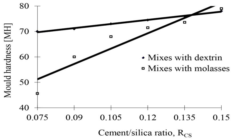
Figure 2: Changes in mold hardness with increasing cement/silica ratio,  $R_{CS}$ .
