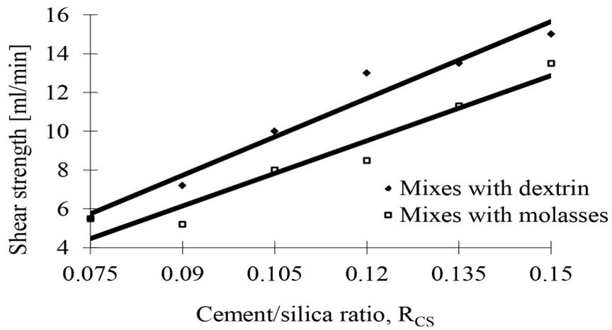
Figure 6: The shear strength profile with increasing  $R_{CS}$ .
