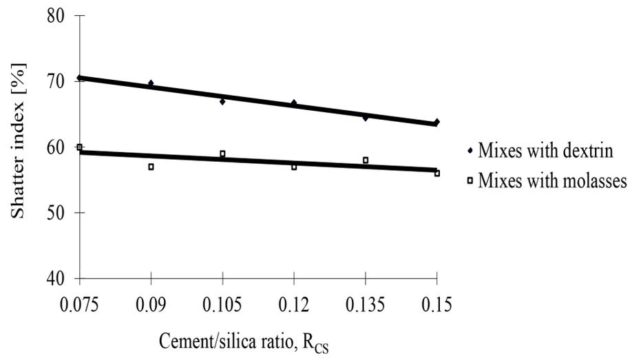
Figure 4: Shatter index versus  $R_{CS}$  for different additives.
