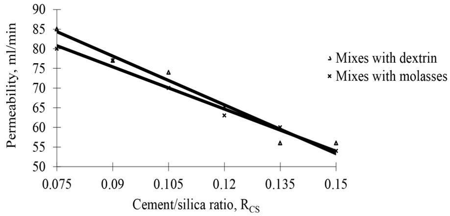
Figure 3: The changes in permeability with increasing  $R_{CS}$ .
