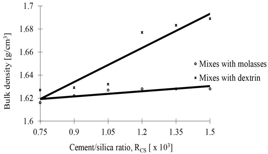
Figure 1: Changes in the bulk density with increasing cement/silica ratio,  $R_{CS}$ .
