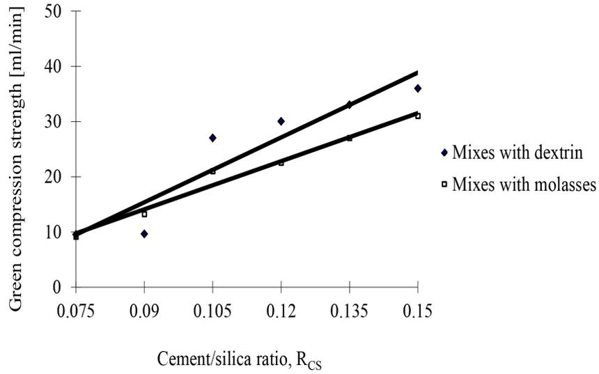
Figure 5: The green compression strength profile with increasing  $R_{CS}$ .
