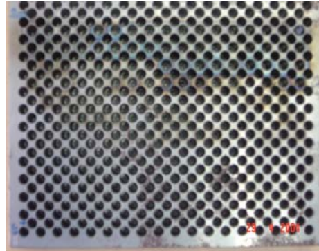
Figure 2: Medium carbon alloy steel work piece after 473 drilled holes
