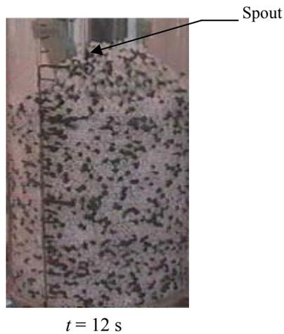
Figure 9: Photograph showing the spout of homogeneous mixture at bed depth of 17 cm and gas velocity of  $1.38 U_{mf}$ .
