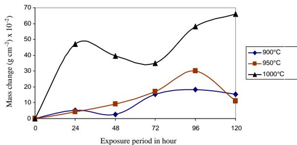
Figure 1: The change in mass with time (oxidation kinetic) curves of stainless steel AISI 304 coated with MgCO<sub>3</sub>, oxidized at 900°C, 950°C and 1000°C.
