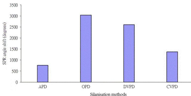
Figure 3: Amine accessibility for various silanisation methods.
