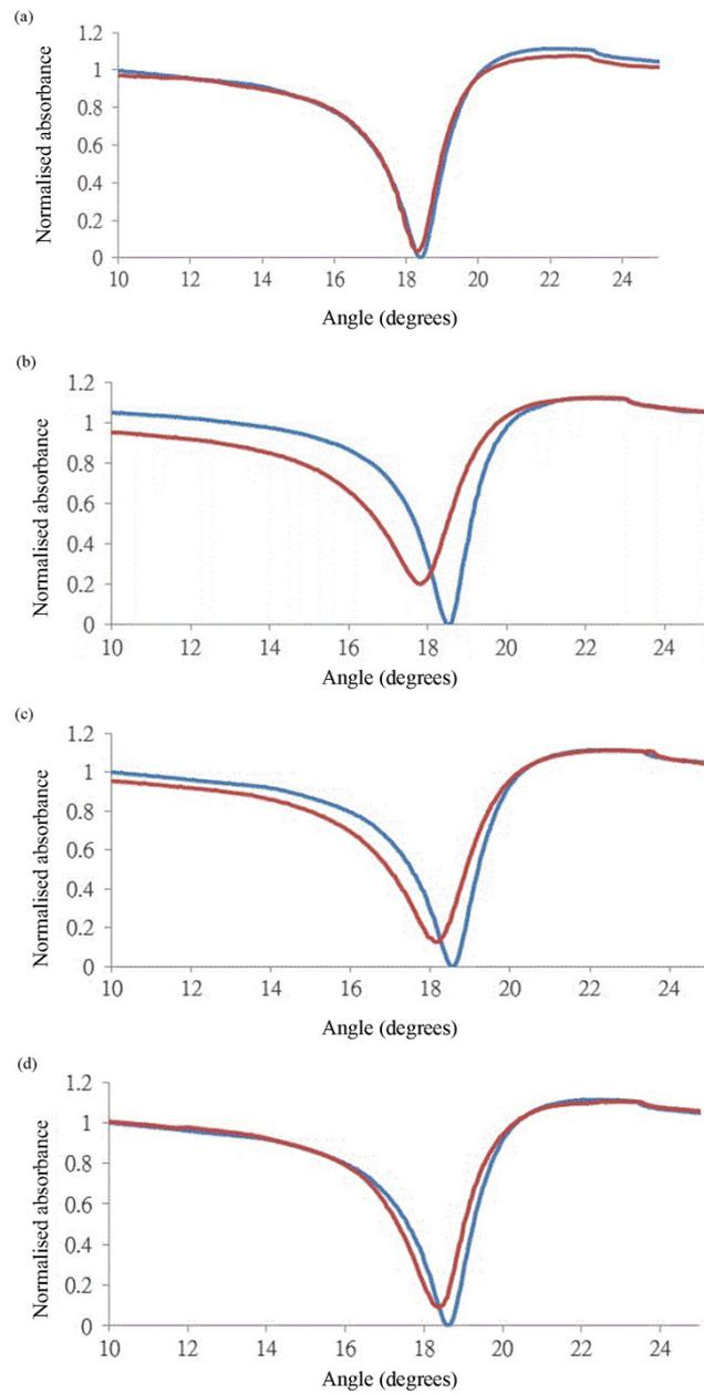
Figure 2: SPR response of sputtered thin Au/Ag films silanised with APTES by (a) APD, (b) OPD, (c) CVPD and (d) DVPD methods.
