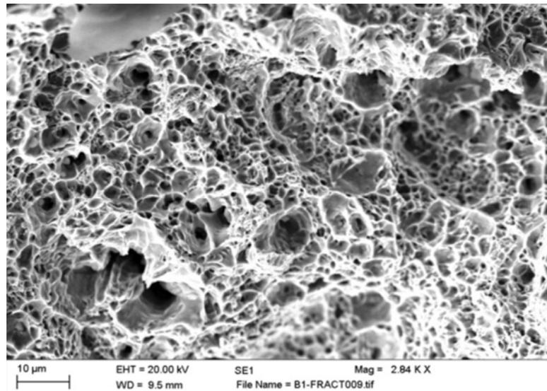
Figure 2: SEM structure of sample B-1 showing ferrite-martensite pull-out.
