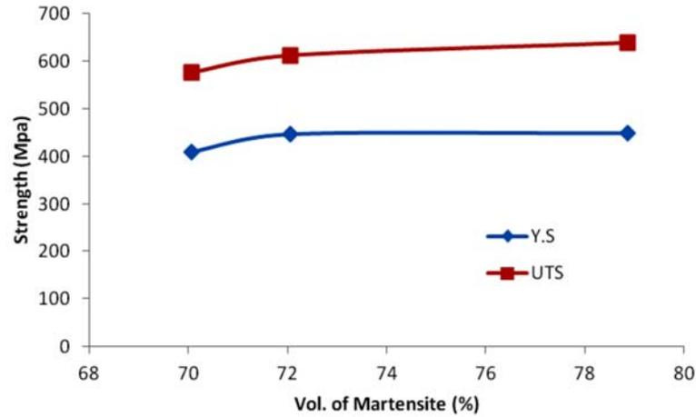
Figure 1: Variation of strength with volume in the martensites.
