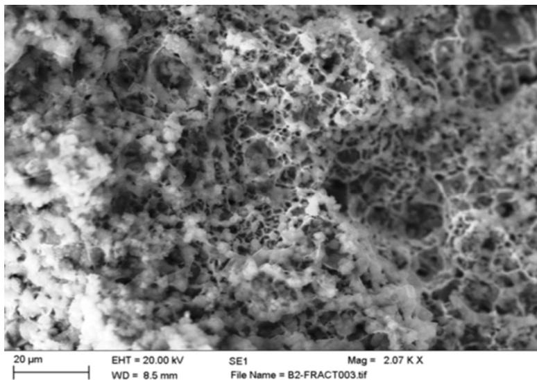
Figure 3: SEM structure of sample B-2 showing ferrite-martensite colonies.
