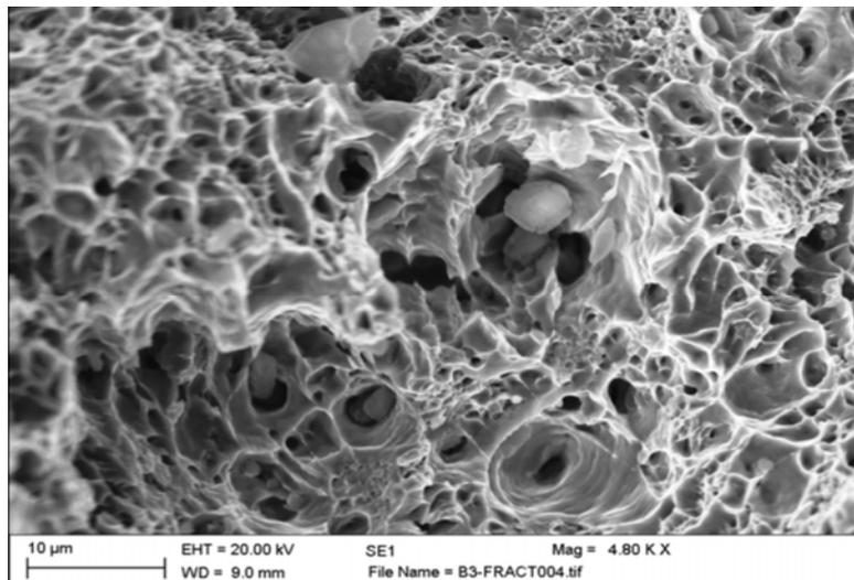
Figure 4: SEM structure of sample B-3 showing intermetallic compounds amidst ferrite-martensite pull-outs.
