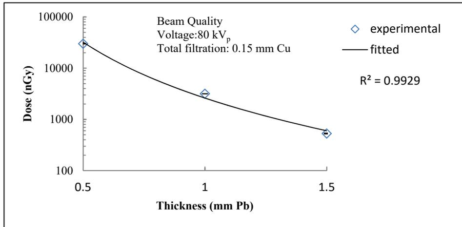
Figure 4: Relationship between reference lead thickness and measured dose at X-ray tube voltage of 80 kV<sub>p</sub>.
