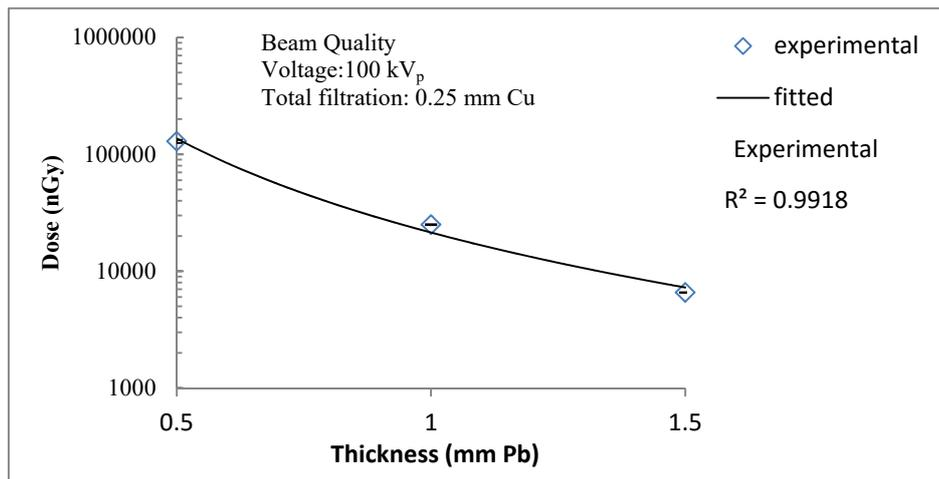
Figure 5: Relationship between reference lead thickness and measured dose at X-ray tube voltage of 100 kV<sub>p</sub>.
