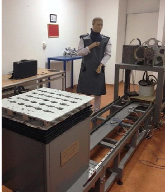
Figure 1: A photograph of a radiometric bench used for measurement of attenuation properties of X-ray protective materials.
