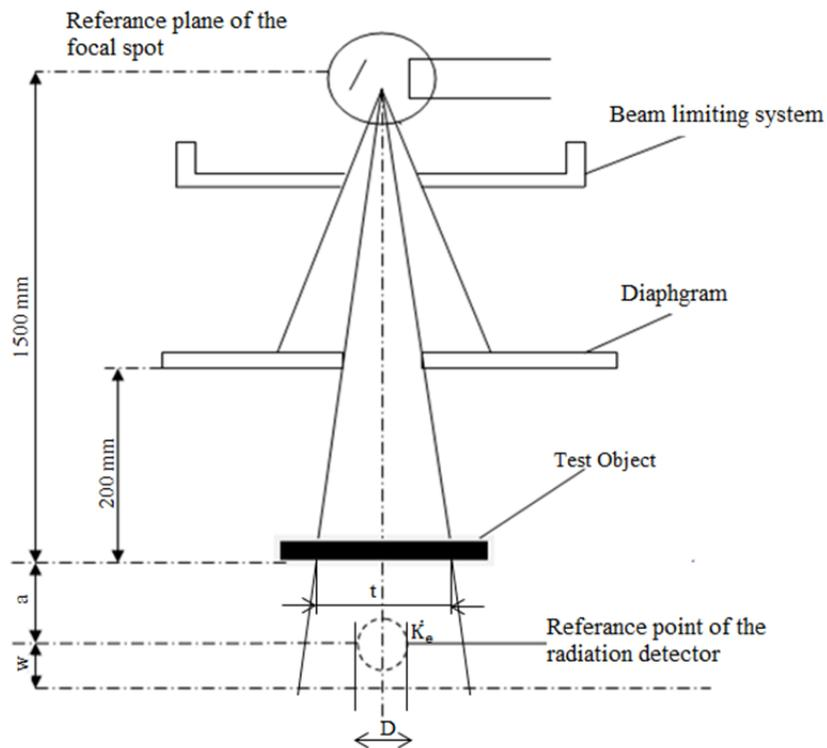
Figure 2: Narrow beam geometry, NBG.<sup>4</sup>
