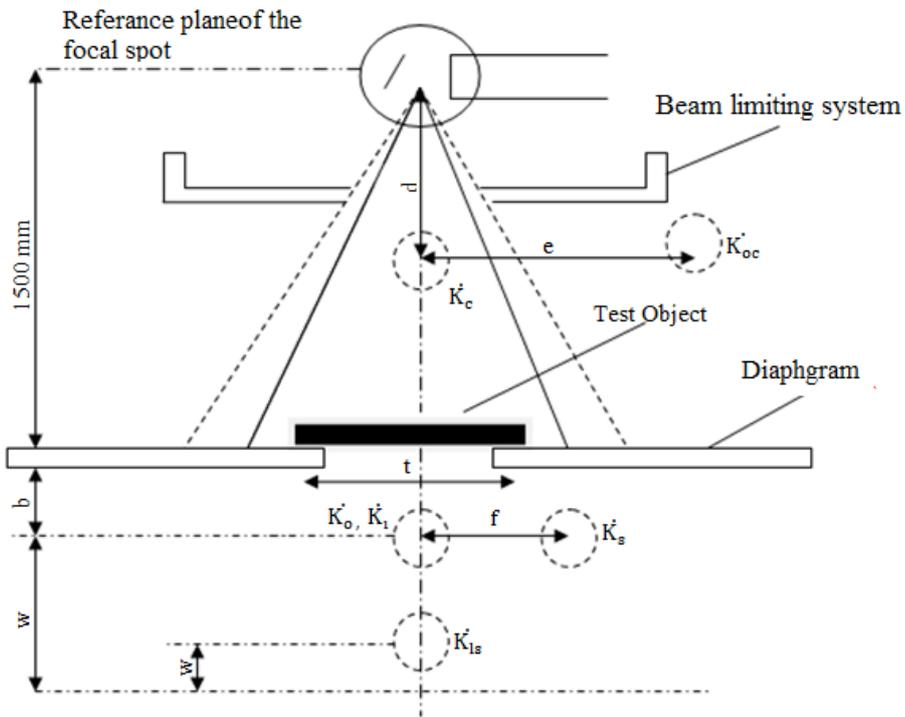
Figure 3: Broad-beam geometry (BBG).<sup>4</sup>
