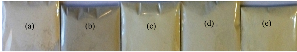
Figure 1: Photography of the parent bentonite (a), and ion exchanged bentonite with copper sulfate for 10 min (b), 20 min (c), 40 min (d) and 60 min (e).
