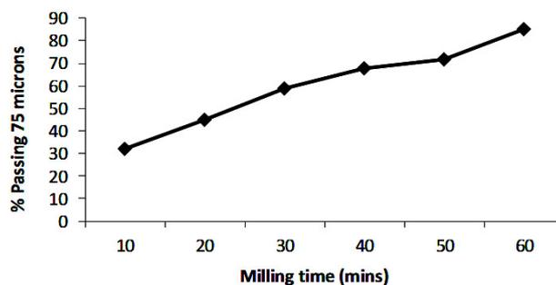
Figure 1: Milling curve for Palabora copper ore.
