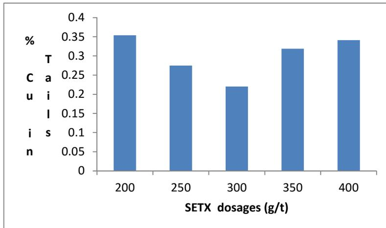
Figure 7: Grade of tailings at varying SETX dosages.
