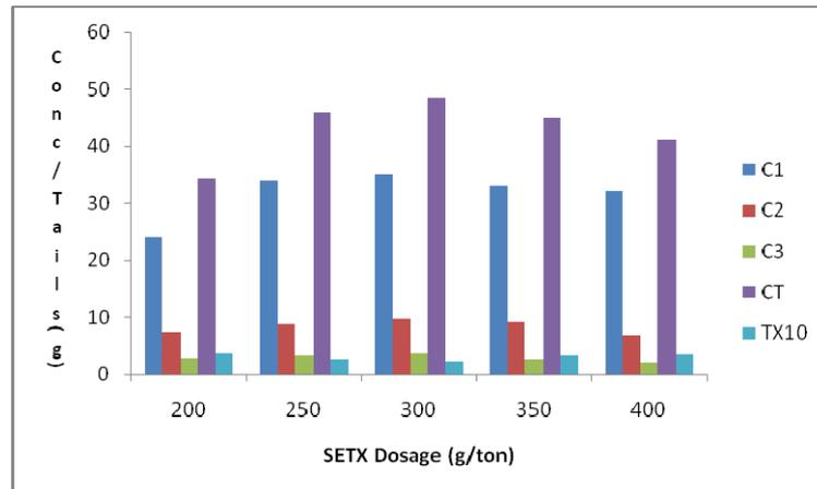
Figure 3: Weights of Cu concentrate (C1, C2, C3, CT) and tailings (TX10) obtained at varying scraping times and SETX dosages.
