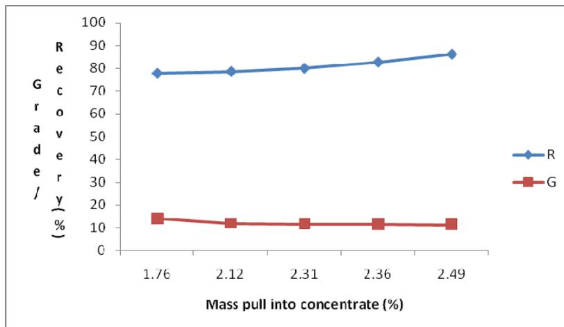
Figure 5: Grade and recovery (%) at varying mass pull (%).
