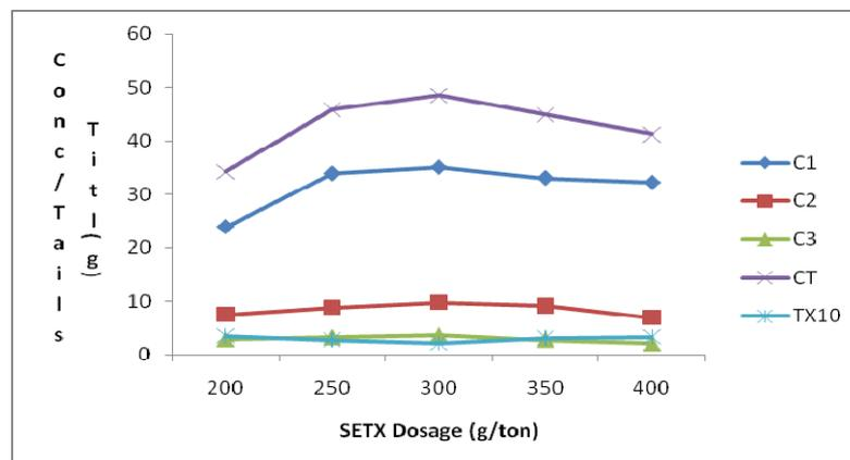
Figure 2: Weights of Cu concentrate (C1, C2, C3, CT) and tailings (TX10) obtained at varying scraping times and SETX dosages.
