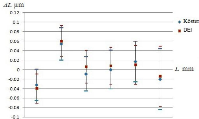
Figure 6: Results obtained by the DEI and Köster comparator for a set of 6 gauge blocks of length (2 mm, 5 mm, 10 mm, 20 mm, 25 mm, and 75 mm) show good agreement.
