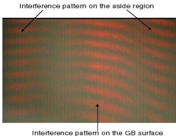
Figure 3: Interference fringes on gauge block surface and the aside region resulted from the superposition of the beams reflected from interferometer arms (measuring arm M1, M2, gauge block and reference arm M3).
