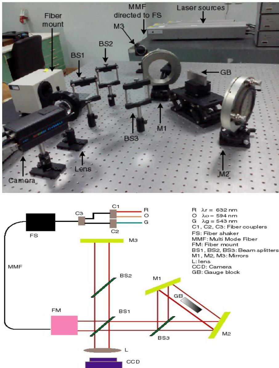
Figure 1: Optical system setup (above) and schematic diagram (below).
