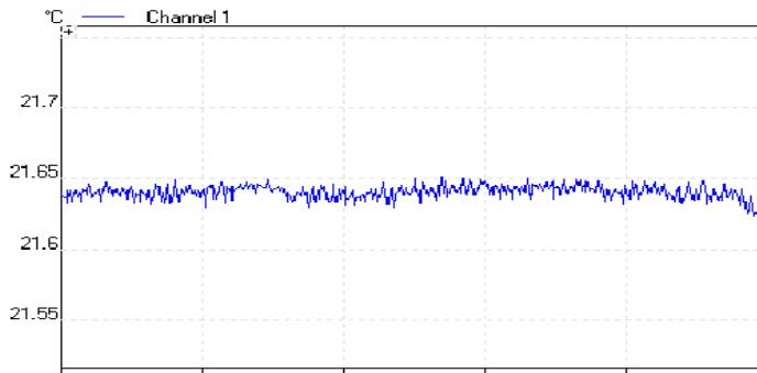
Figure 5: Gauge block's temperature display for 3 h shows good stability of the gauge block in the interferometer.
