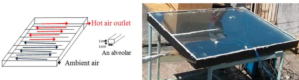
Air circulation within the polyethylene plate
