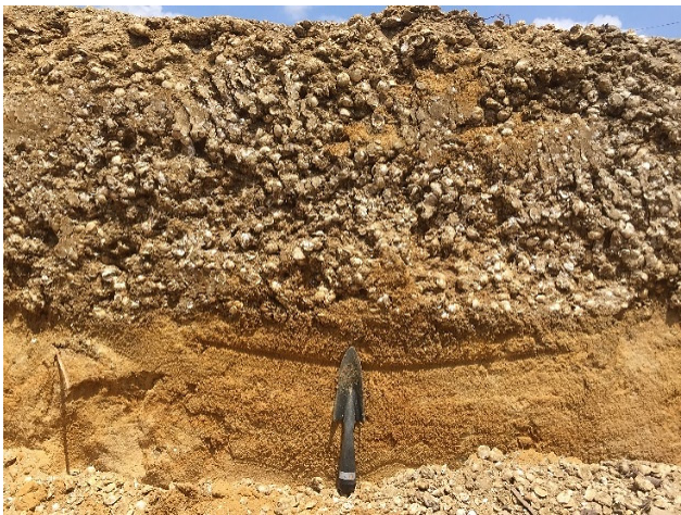
Figure 3: Compacted shell layer in sandy-clay soil overlying sandy layer.
