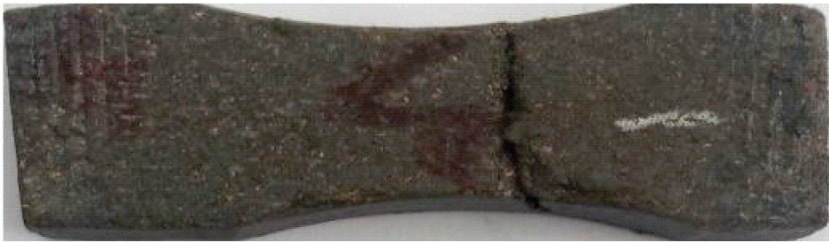
Figure 4: Friction material specimen after tensile testing showing failure.
