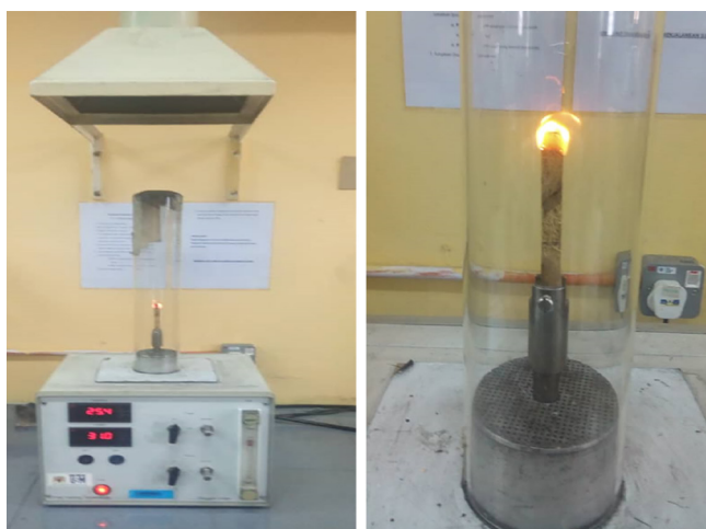
Figure 1: LOI experimental set-up.
