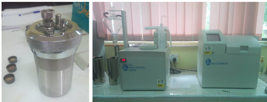
Figure 2: Bomb calorimeter experimental set-up.
