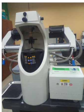
Figure 3: DMA experimental set-up.
