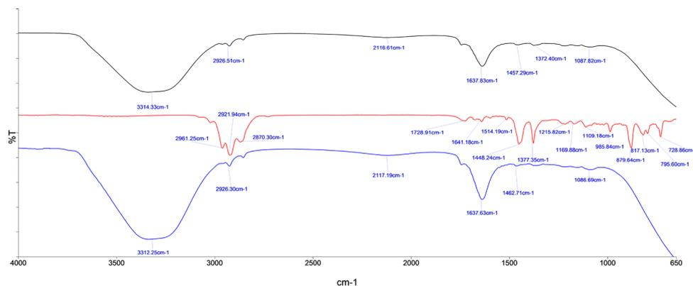
Figure 4: FTIR spectroscopy of ZOE (red), nanostructured lipid carrier (blue) and NLC-ZOE formulation (black).
