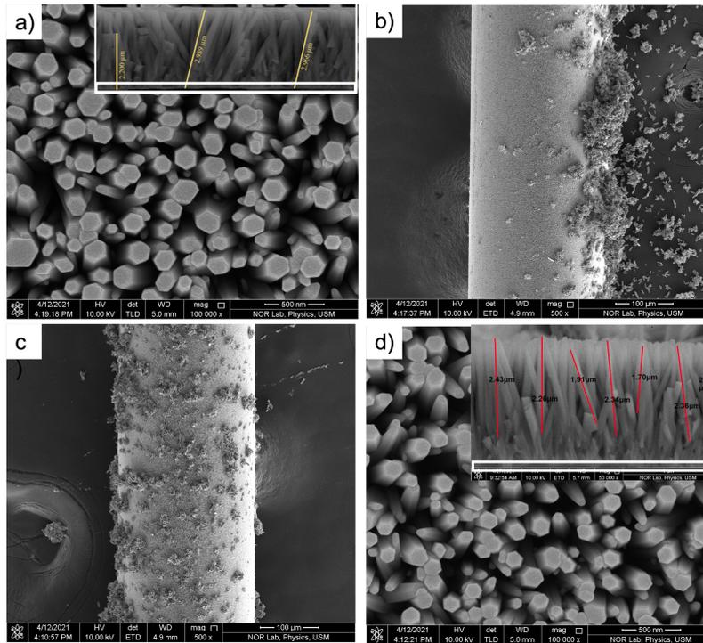
. Figure 2: FE-SEM images of the gain medium, ZnO microstructures, prepared on optical fibres where (a) is top view image at 100k magnification with inset showing the cross section of the microrods for Sample 1, (b) is top view of the fiber for Sample 1, (c) top view of fibre for Sample 2 and (d) top view of the microstructures with inset showing the cross section of the microrods for Sample 2.
