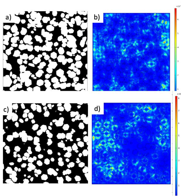
Figure 8: Simulation of light propagation within the structure of Sample 1 and Sample 3 whereby (a) and (c) refer to the FE-SEM images of Sample 1 and Sample 3, respectively; (b) and (d) refer to the light confinement from Sample 1 and Sample 3, respectively.
