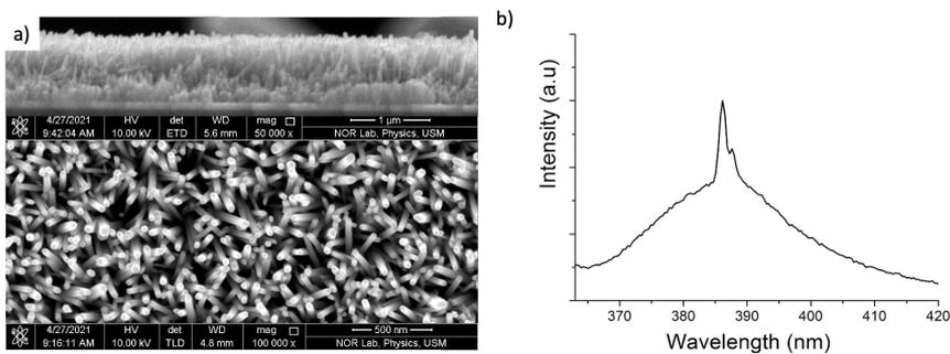
Figure 7: (a) FE-SEM image of the ZnO nanorods with upper figure showing the cross section and the bottom figure shows top view and (b) random lasing emission from the ZnO nanorods prepared on glass substrate.
