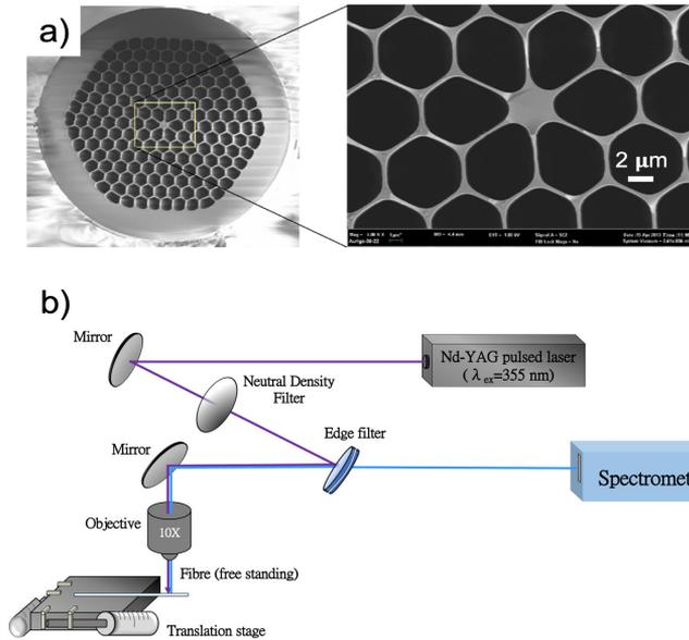
Figure 1: (a) Structure of the PCF, (b) The PL setup for random lasing measurement: The pump light was focused using a 10× objective onto free standing fibre placed on a translational stage.
