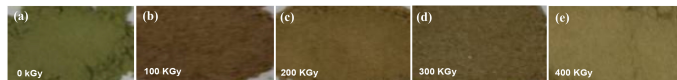
Figure 1: Optical images of WH biomass powder after EBI pretreatment at (a) 0 kGy, (b) 100 kGy, (c) 200 kGy, (d) 300 kGy and (e) 400 kGy.
