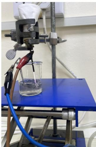
Figure 1: Synthesis of ZnO NPs by plasma jet.
