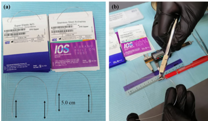
Figure 1: Samples (a) were obtained by cutting both distal ends of each archwire (see [b]).
