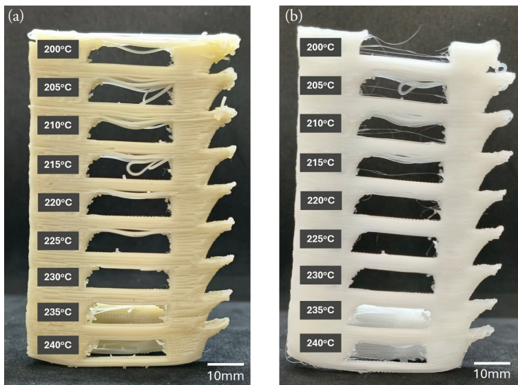
Figure 6: Temperature tower printed with (a) rHDPE and (b) commercial HDPE filaments.
